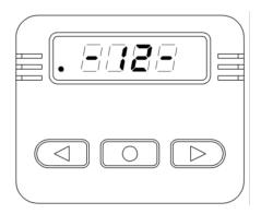
If the Temperature Control mode is selected (regardless of activation of the Ventilation mode), then the required value of temperature is set by pressing the buttons (decrease) or (increase) (in the range from 1 to 30°C in the zone of the selected
