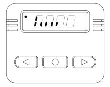
If the Heat Control mode is selected, then the required value of heating power is set by pressing the buttons (decrease) or (increase). An 8-step scale is displayed
